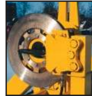
Bronze disc brake with hydraulic caliper (in lieu of manual caliper)
