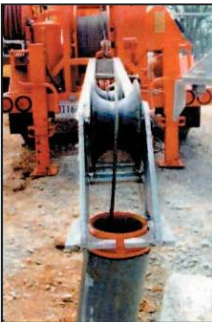
Optional 3 roller assembly (stinger) to provide a larger bending radius.
