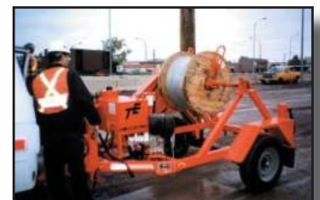
Hydraulic tensioning reel stand, skid based or trailer mounting
