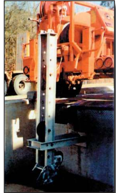
The jib is positioned with quick change pins, no tools are required.
