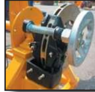
Bronze disc brake with manual caliper
