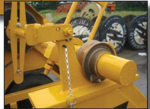
Bronze outer bearing support with quick pin released locking latch
