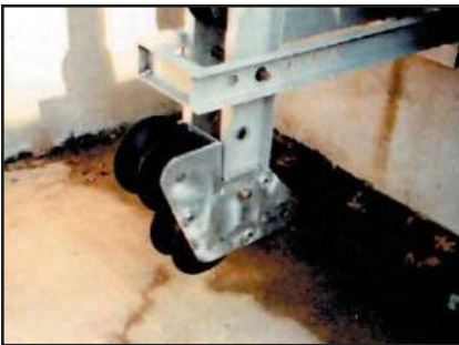
Optional 3 roller assembly (stinger) to provide a larger bending radius.
